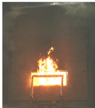
Figure 4: Fire emitting from the test window
